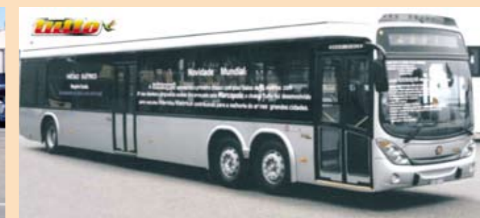
15m Tutto Chassis, 2nd drivable front axle with low floor for applications on hybrid tractions that use renewable fuels (alcohol, NVG, biodiesel and hydrogen)
